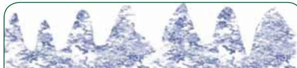
Untreated surface of glass as seen under a microscope.
